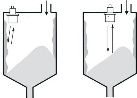
When you mount the transducer on the solid tank, the transducer must point to the tank outlet.
