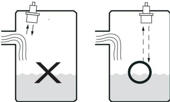
The transducer should not be mounted too close to the tank wall, the bracket can cause strong false echoes.
